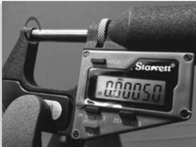
A Starrett micrometer is used to measure a sheet of stainless steel, which, at 0.0005 inch thick, is thinner than paper. Brewster Washers uses the sheet to make a thin washer to precisely level missile guidance systems. The washer is in the upper left corner of the photo. Photo courtesy of Brewster Washers.
