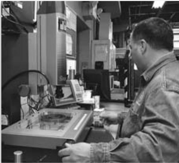
Brewster Washers President Sal Freda, Jr., demonstrates a measuring device used in the plant to measure the precision of a company's part. The metrology department appears to have six measuring devices ready for use, as well as historic hand-held micrometers. Photo by Mark Langlois.
