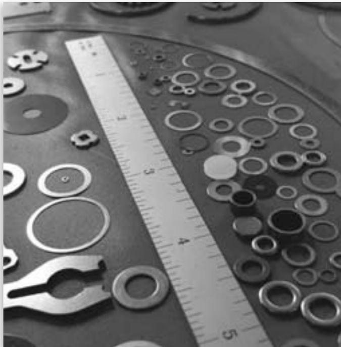
Various washers manufactured by Brewster Washers, Fairfield, N.J. The company uses numerous materials—including copper, brass, aluminum, cold rolled steel, phosphor bronze, stainless steel, and non-metallic materials—to make the washers. Photo courtesy of Brewster Washers.
